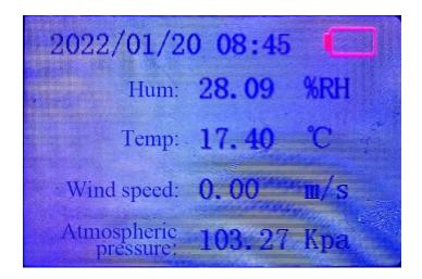
After the handheld weather station is turned on (click "on"), the main interface of the system will be displayed as shown in the figure above. The interface displays the current time and the real-time weather values collected by each sensor. The battery symbol shows the remaining power of the system.
