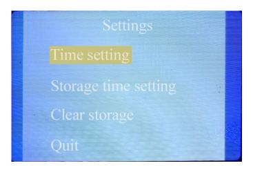
Click the SET button in the main interface of the system to enter the setting page as shown in the above picture, which includes setting the time, setting the storage time, clearing the storage and exiting the setting page respectively.
